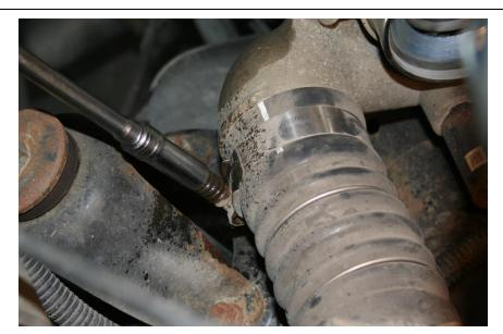
11.Pry off the metal lock from rear manifold bolts, remove the heater pipe bracket from the bracket.
