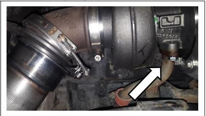
14.Install the oil supply line (reuse OE line).
