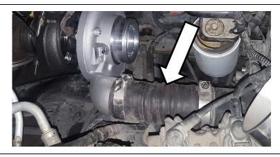
16. Connect the exhaust to the downpipe. Tighten clamp.
