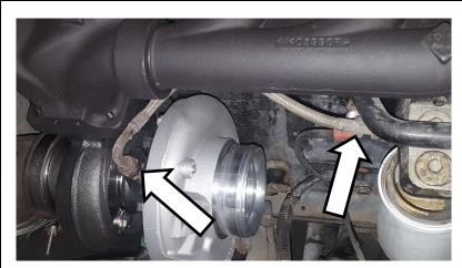
15. Connect the CAC pipe and boot to the turbo charger. Tighten clamps.
