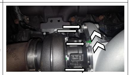
12.Install the supplied (1453152) oil supply fitting onto the turbocharger with a light amount of thread sealant.
