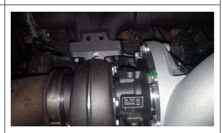
10.Check that there is approximately 1/4" clearance between turbo and shock tower. Clock turbo if required, see step 10.
