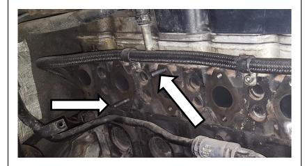
2. Install 4 supplied 25mm M10 studs onto the T4 flange. Use the 1/8NPT plugs to block the port on the manifold if not being used.
